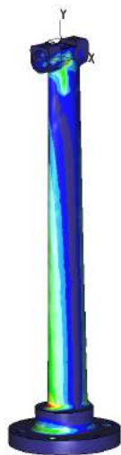
Figure 3. Finite-element results showing von-Mises stress for lightly-loaded case (1 Nm input torque).
