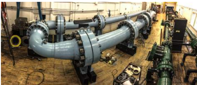
Figure 1. The High Reynolds Number Test Facility (HRTF) at the Princeton Gas Dynamics Laboratory. Direction of flow is clockwise from above.
