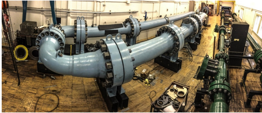
Figure 2.1: Photograph of the high-pressure wind tunnel known as the HRTF (in blue).
