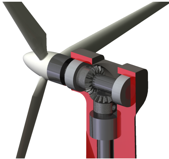
Figure 2.7: Computer rendering of the HAWT tower assembly with prototype rotor geometry for reference. Cut-away detail shows the internal gearbox geometry.
