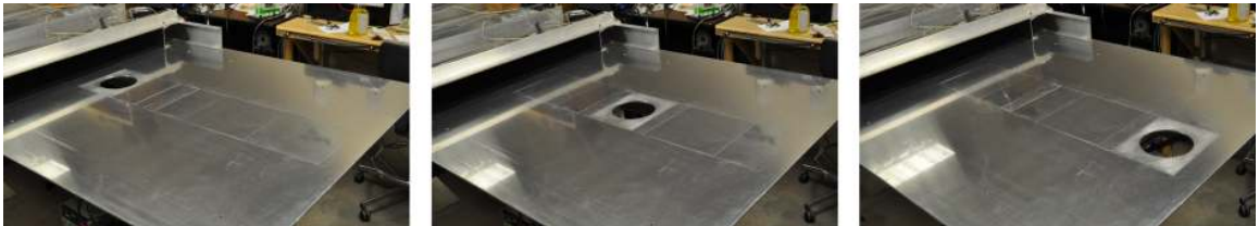
Figure 3.8: New modular test section floor, with measurement instrumentation plug holder at three streamwise positions (actual instrumentation plug not pictured).
