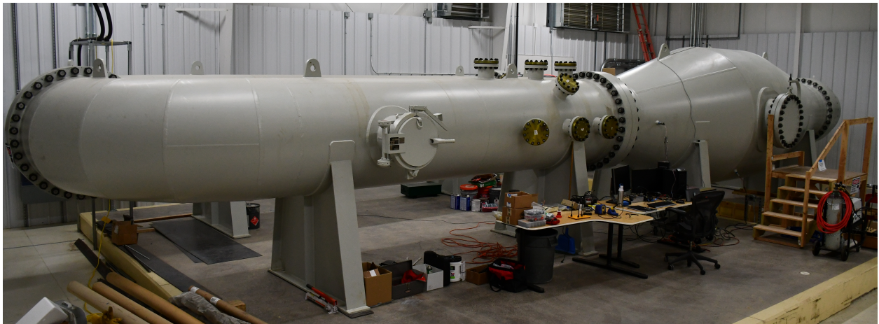
Fig. 3 The Compressed Air Wind Tunnel (CAWT), a low-speed, closed-loop wind tunnel in which the internal ambient pressure can be raised to 34 atmospheres.
