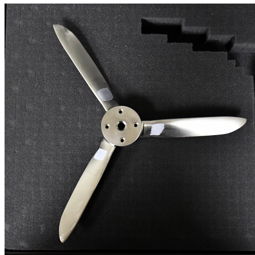
Fig. 5 The small-scale, fixed-pitch UAM rotor used to collect data for high Reynolds numbers in the CAWT.
