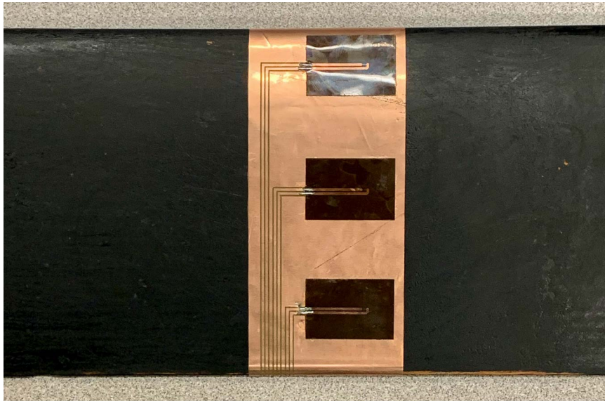
Figure 3.3. Hot-film prototype fabricated for use in experiments attached to an NACA 0012 airfoil. The copper substrate wraps around the leading and trailing edges. Sensor leads are concealed on the opposite surface of the airfoil and extend away from the array towards the airfoil root, where they are connected to driving circuitry.
