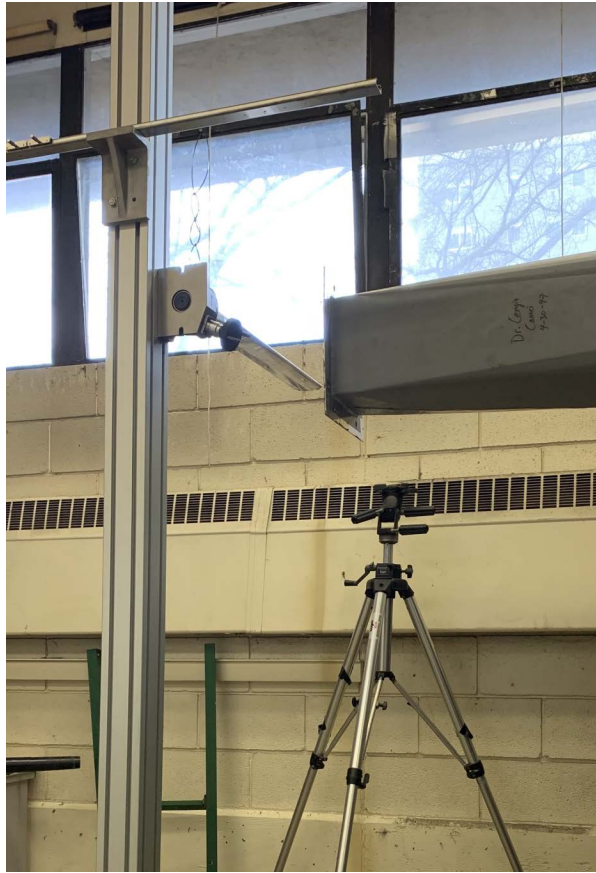
Figure 4.4. The barebones version of the open-jet wind tunnel setup, containing only the airfoil, rotary table, and wind tunnel outlet.
