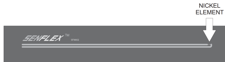
Figure 3.1. Senflex ® SF9902 is a single-element hot film sensor on a 120 mm x 20 mm substrate. Figure reproduced from of Systems Integration Inc. (3) pg. 5.
