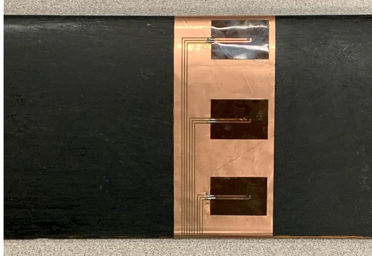
Fig. 4 Linear array hot-film attached to the NACA 0012. The substrate is conformed around the leading and trailing edges of the airfoil. Sensor leads are concealed on the opposite surface of the airfoil extending away from the array to the root and are connected to driving circuitry. A matte black surface treatment is applied to the area surrounding the array to reduce reflections during particle image velocimetry.
