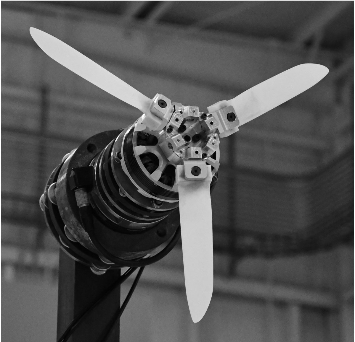
Figure 2.4. The 3D printed rotor blades mounted on a variable-pitch hub machined out of aluminum.
